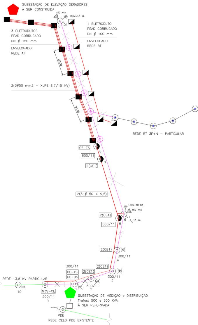
PL. BAIXA - LAYOUT DA REDE DE AT PARTICULAR - A SER REFORMADA SEM ESCALA
